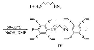
The reaction is accompanied by formation of a large amount of polymer as side product for compound **I** with four vinylthio groups is prone to thermal polymerization [8]. The reaction does not go at 50–60°C. We did not detect any monosubstituted products from a single molecule of compound **I**.
